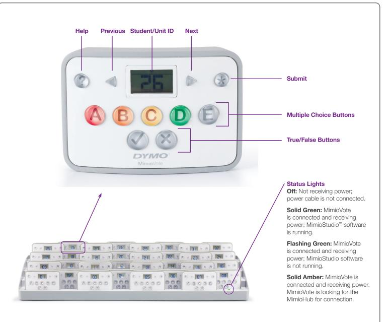
The MimioVote<sup>™</sup> assessment system includes a charging station that also stores all of your MimioVote units. You can place any unit into any slot on the station, and it will automatically be assigned the number for that slot. No need to match a particular unit to a particular slot!
